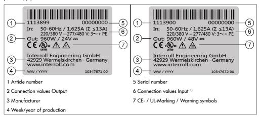
$^{1)}\Sigma \leq$  13 A - When looping through the supply line to a maximum of eight power supplies expected maximum total current.
