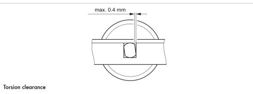
If necessary, install a support plate above the mounting bracket to secure the drum motor axle. However, ensure that the axle remains movable to one side to compensate for thermal expansion.
