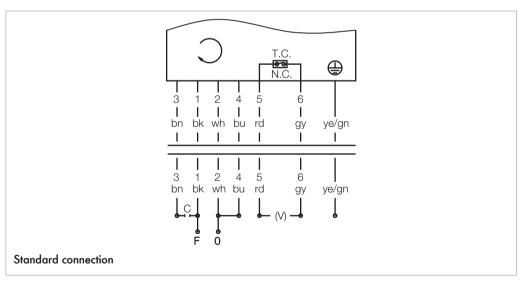
Thermal protection as an option. For a drum motor without thermal protection, cores 5 and 6 are dummies.
