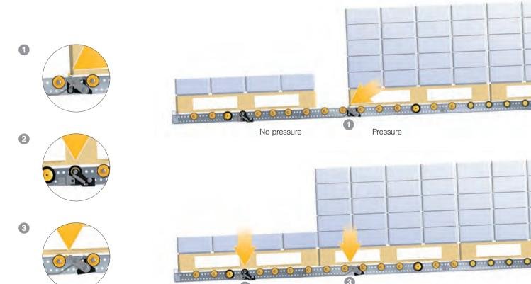
Pedal and separator device on low position simultaneously: no damage
